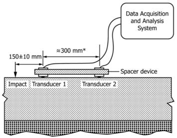
\*Measure to nearest 1 mm the actual distance between centers of transducers FIG. 1 Schematic of Testing Configuration for Procedure A
