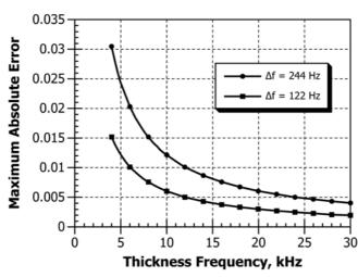
FIG. 8 Maximum Systematic Error Due to Frequency Interval as Function of Thickness Frequency
