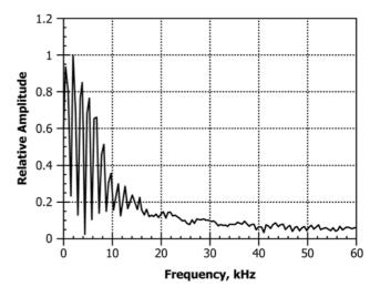
FIG. 6 Example of Invalid Impact-Echo Test, Waveform Does Not Display Periodic Oscillations and Amplitude Spectrum Does Not Have Single Dominant Peak
