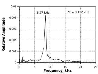
FIG. 5 Waveform and Amplitude Spectrum for Valid Impact-Echo Test of 250-mm Thick Concrete Slab
