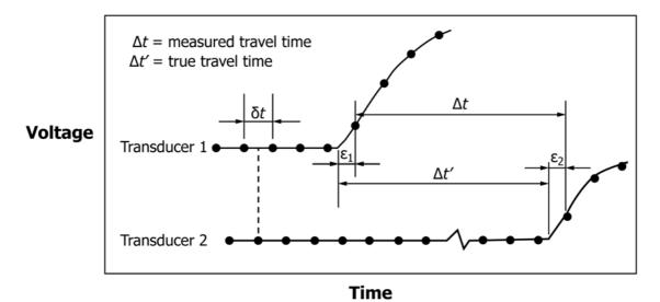
FIG. X1.2 Schematic of Early Part of Waveforms Obtained from Procedure A With a Data Acquisition System That Samples Each Channel Alternately
